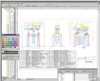
SolidWorks automatically creates production-level drawings (any combination of views) from a model, such as this assembly with a bill of materials included. Additional views can be added easily.
