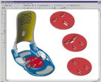
Using SolidWorks, configurations of products, assemblies, and product families can be created and managed from the original design, such as the multiple bolt patterns shown here for a snowboard binding.
