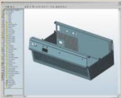
Specialized functionality, such as built-in SolidWorks sheetmetal features, can be an important consideration for manufacturers that are migrating to 3D. SolidWorks also offers modules for piping and mold base assembly.
